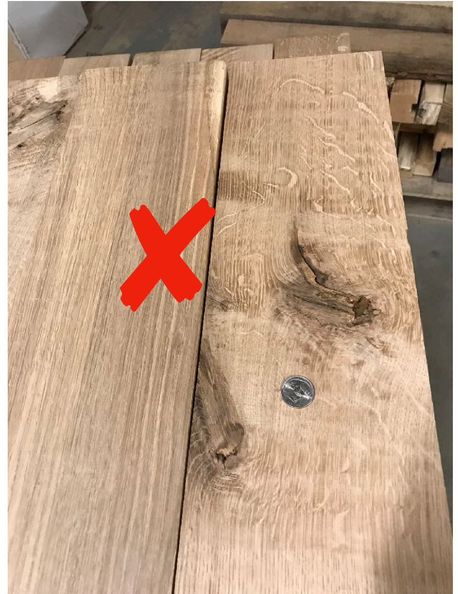
Defect out even if middle of board 2 Knots + 2 Close = Defect
