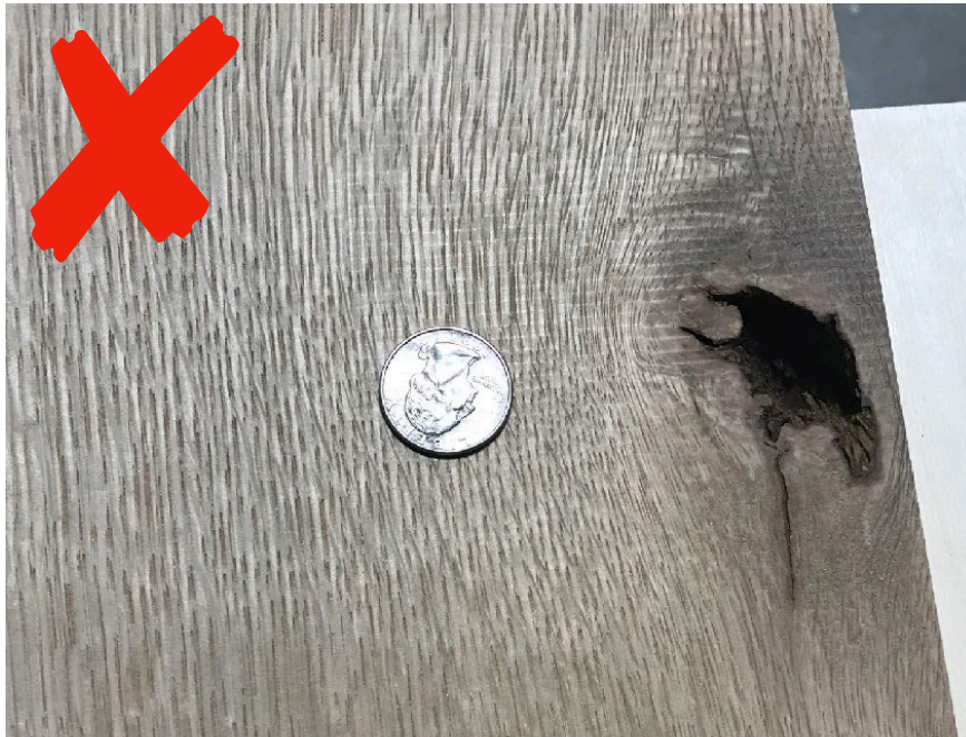
Defect out open holes larger
