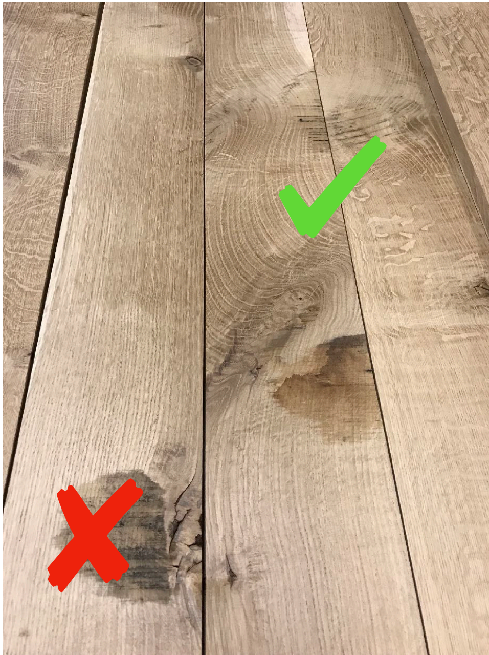
Defect side knot, swirl/figure ok
